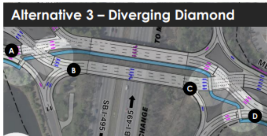
Caption: Alternative 3 - Diverging Diamond highlights A, B, C and D shared use path crossings, many of which are multilane. Source: MDSHA (Round 2 Design Assessments)
